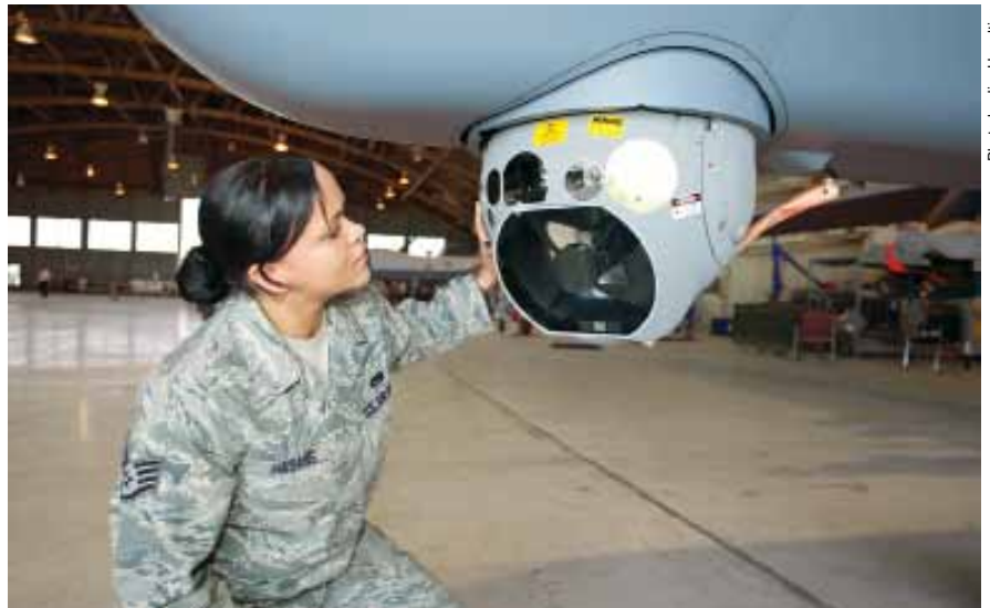
SSgt. Stephanie Hagans inspects the “eye” of a Reaper, the MTS-B Multispectral Targeting System. Plans call for Reaper to supply 10, and then 30, video feeds.
