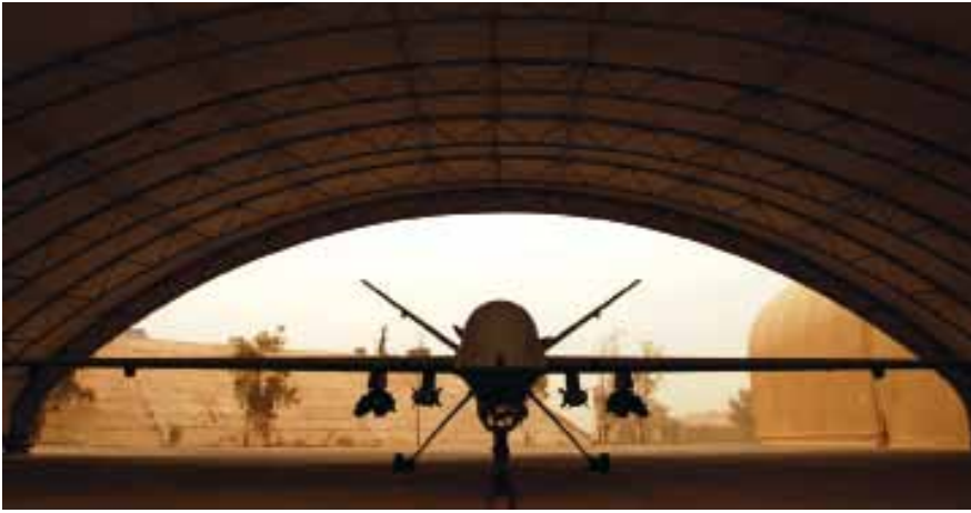
An MQ-9 Reaper takes shelter during a sandstorm at JB Balad, Iraq. A Reaper fitted with Gorgon Stare can pass 10 discrete video feeds to separate users.
